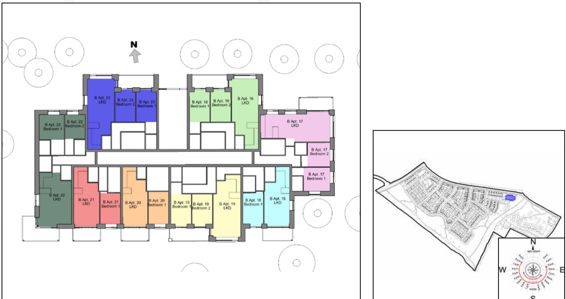
Figure 6.9: Floor plan of assessed building (L), Keyplan highlighting the assessed building (R).
