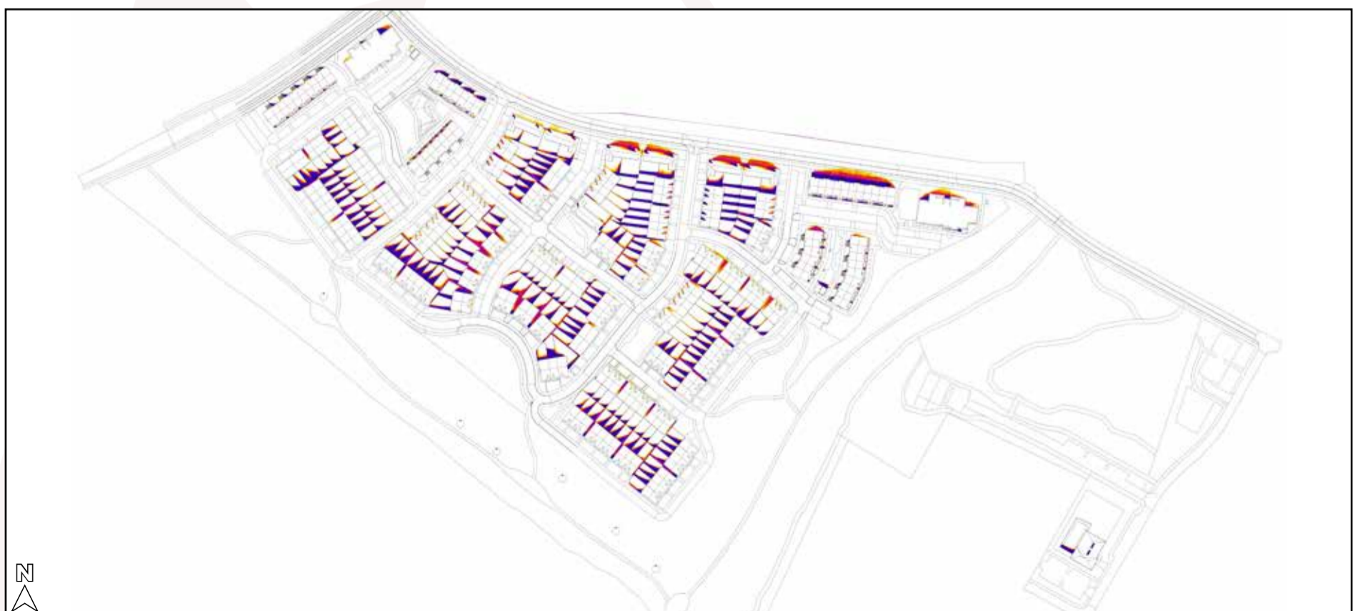
Figure 6.1: Indication of the amenity areas that have been analysed (L), Area capable of receiving 2 hours of sunlight on March 21st shown in white (R).
